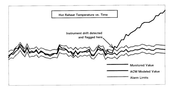
At the left side of the graph, the monitored sensor closely matches **ACM** modeled values and remains well within the dynamic alarm limits. This indicates that the sensor was initially operating properly. But at the right side of the graph, the monitored sensor crosses over the **ACM** alarm limit indicating that the sensor has drifted significantly out of calibration.
