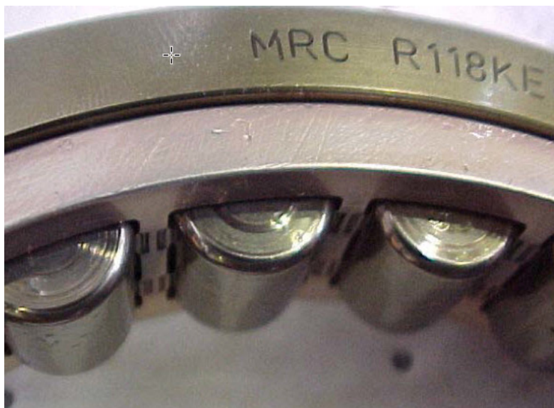
Figure 7: #2 Bearing showing roller end wear
